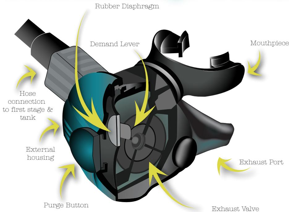
The ability for humans to explore our planet's underwater environment can only be achieved through mechanical means, one of which is SCUBA (Self-Contained Underwater Breathing Apparatus). The second-stage regulator, as shown, is the last phase in the complex and vital air delivery system utilized by scuba divers.
